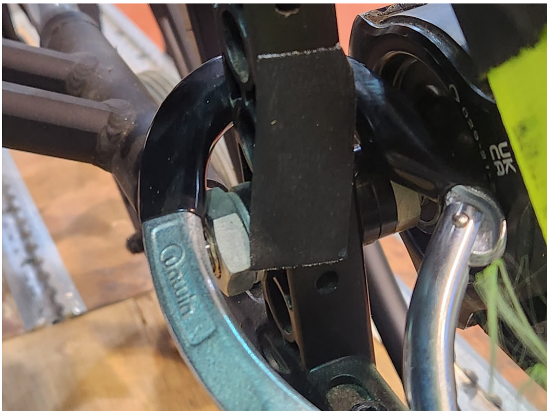
Figure 14: RH inner quick release fixing and RH upper tie-down attachment rear view, pre-test
