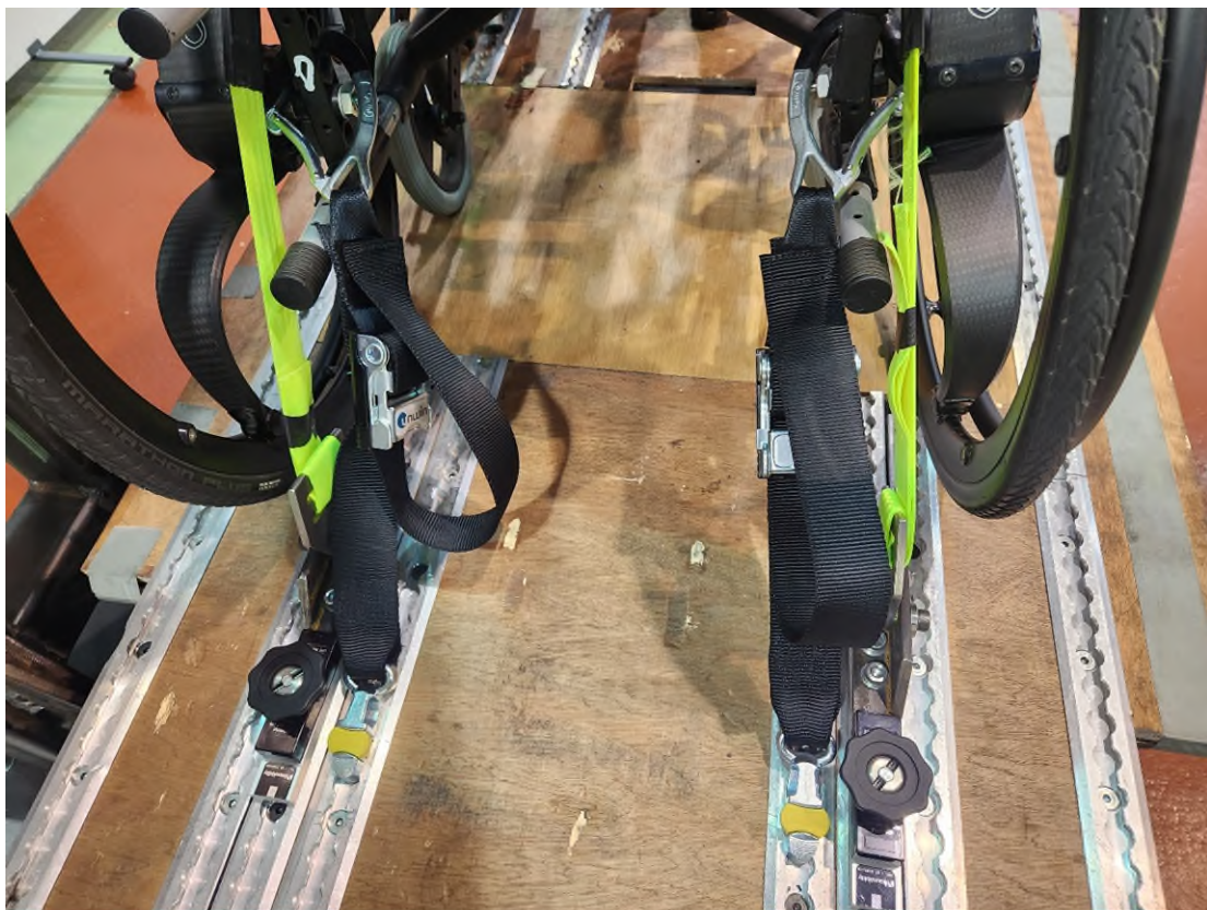
Figure 23: Rear tie downs and ORS anchorage rear view, post-test
