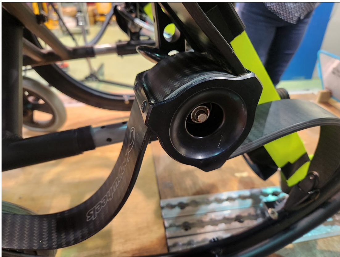
Figure 31: LH wheel quick release mechanism LH side view, post-test
