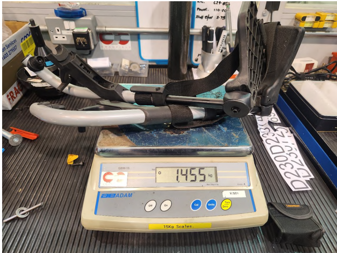
Figure 42: Mass of detached components; 1.455kg, post-test
