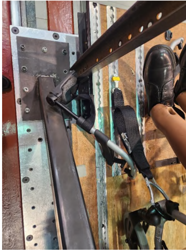
Figure 28: LH foot support top view, post-test
