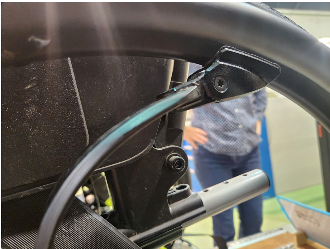
Figure 33: LH upper inner wheel spoke attachment LH side view, post-test
