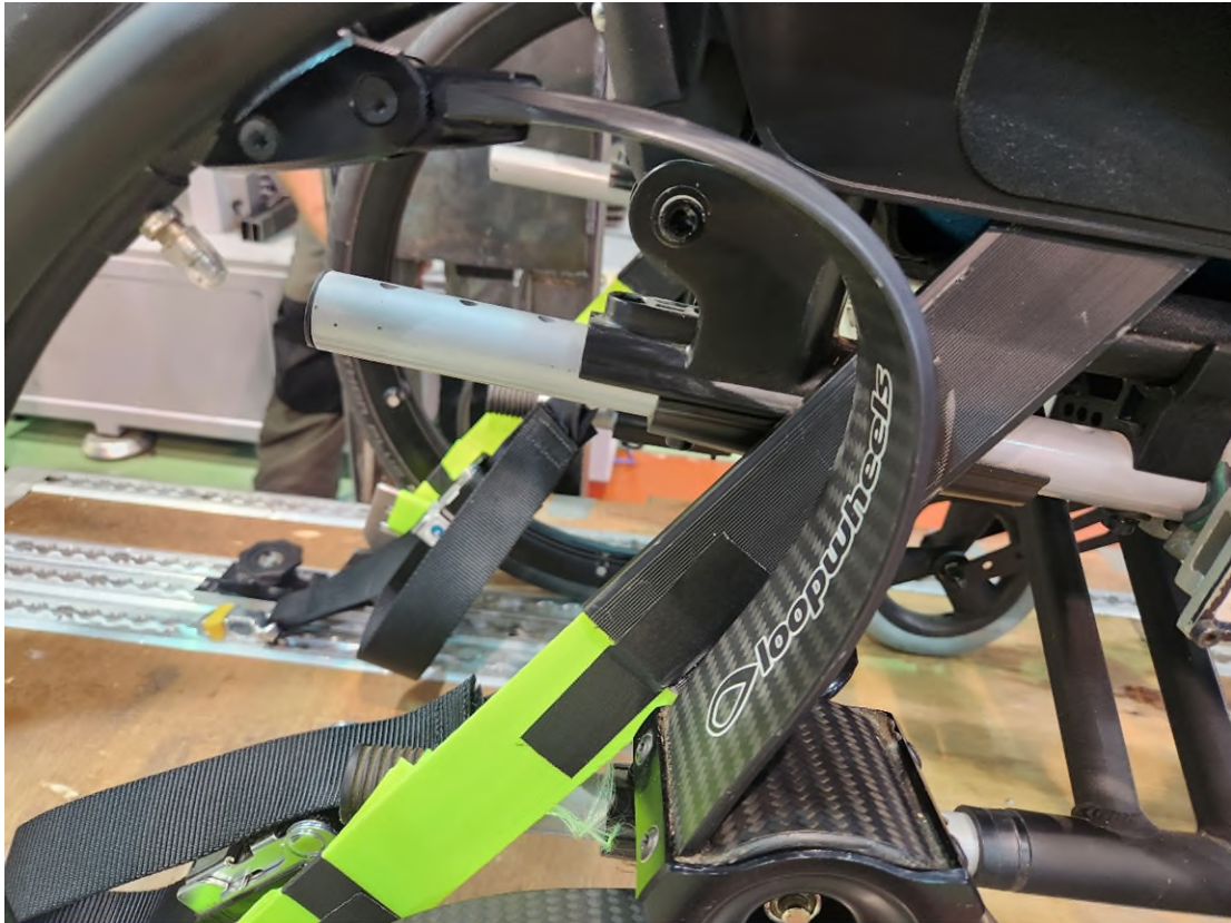
Figure 40: RH rear inner wheel spoke attachment RH side view, post-test
