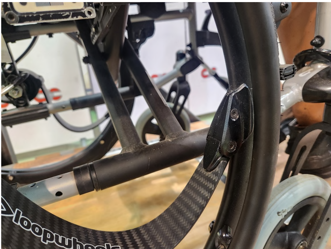
Figure 12: RH inner wheel spoke attachment RH side view, pre-test
