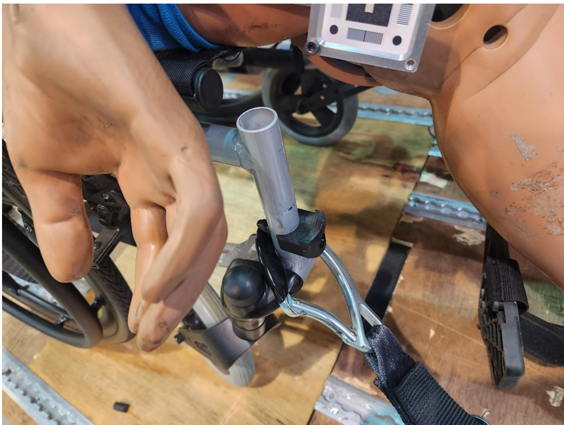
Figure 27: RH foot support attachment point front 3/4 view, post-test
