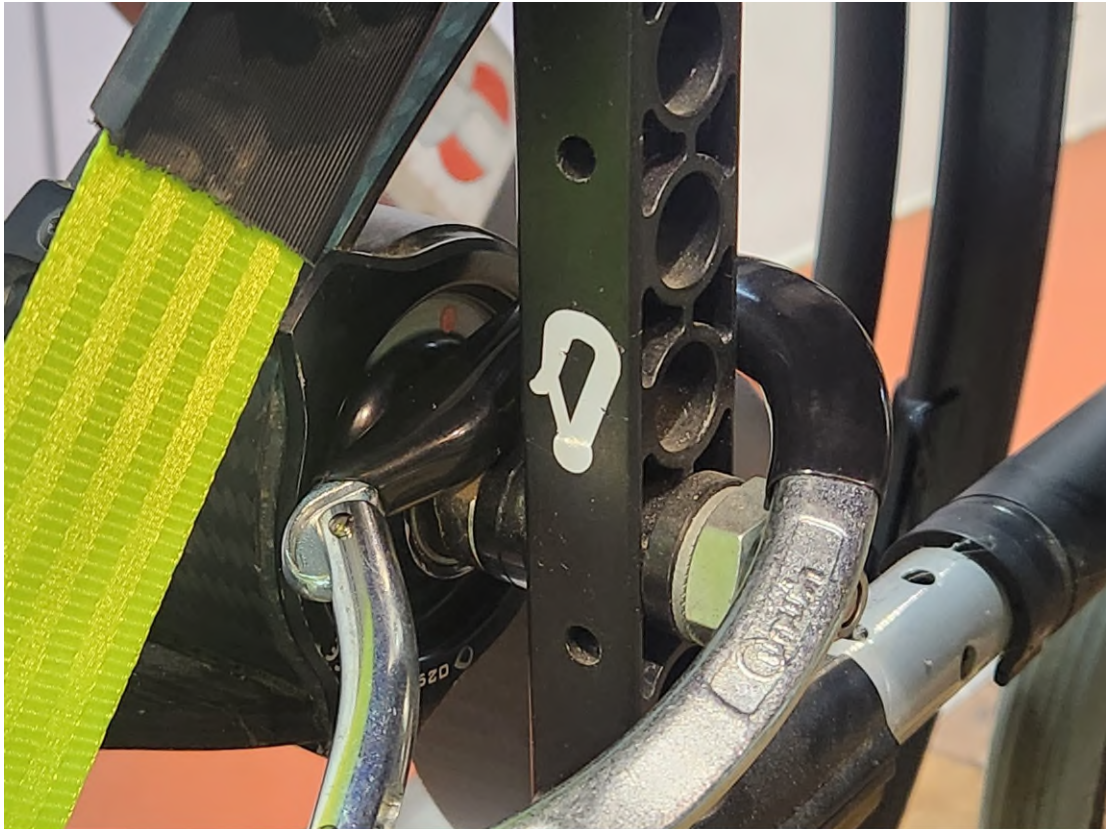
Figure 13: LH inner quick release fixing and LH upper tie-down attachment rear view, pre-test
