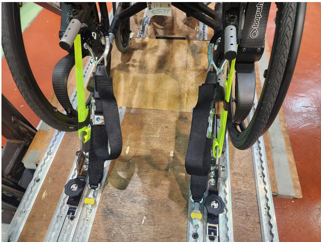
Figure 6: Rear tie downs and ORS anchorage rear view, pre-test
