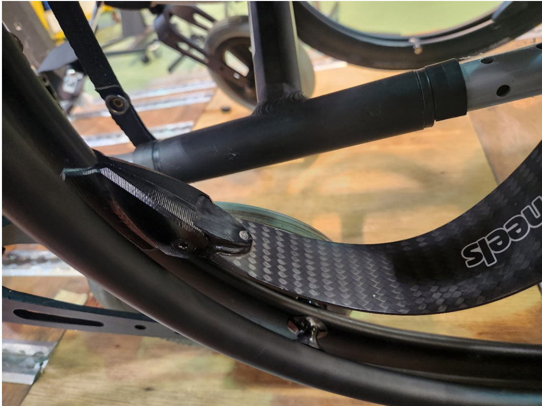
Figure 32: LH front inner wheel spoke attachment LH side view, post-test
