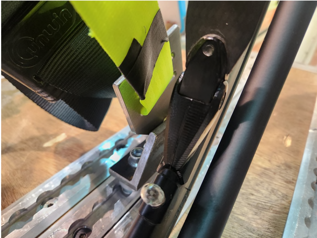
Figure 34: LH rear inner wheel spoke attachment LH side view, post-test
