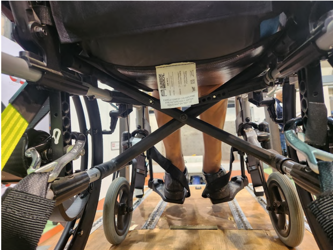
Figure 15: Wheelchair cross brace rear view, pre-test
