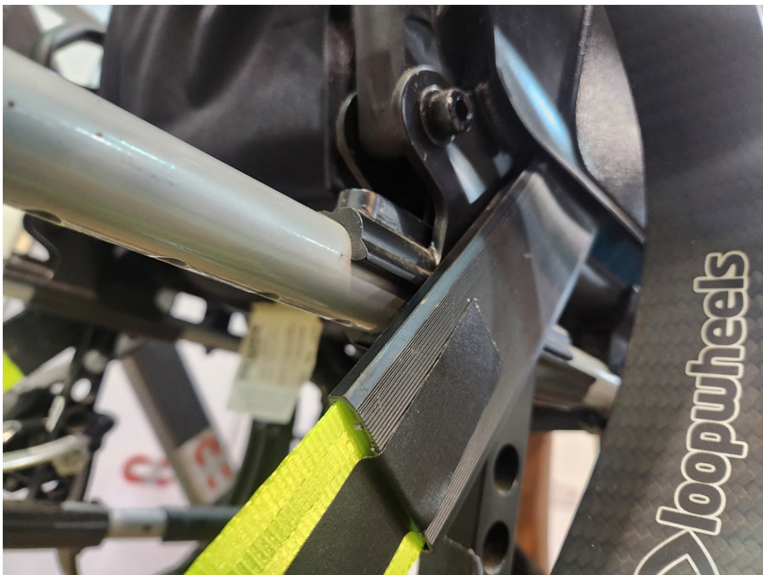
Figure 16: RH ORS routing RH side view, pre-test
