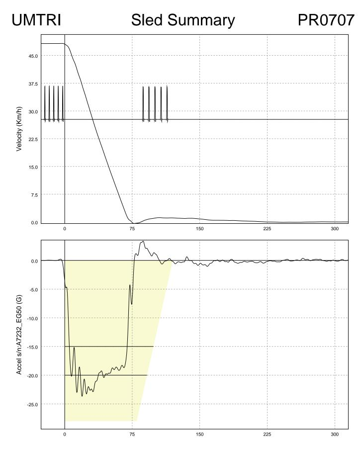
Continuous time under -15.0 G was 64.2 ms Total time under -20.0 G was 26.4 ms Sled Decel Peak = -23.7 G Sled Plateau Average Level = -20.2 G Sled Pulse Duration = 80.4 ms
